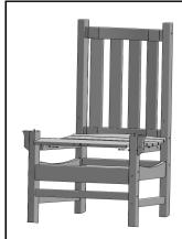
Drop Seat Assembly into seat box in the frame as shown. Secure using (4) 1-1/4" Phillips Head Screws thru the seat supports into the side stretchers of the
