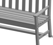
Align counterbored holes in lower side stretcher with Pilot holes in long stretcher,
