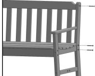
Align counterbored holes in Rear Left Leg with Pilot holes in Back Assembly, ensuring that the
