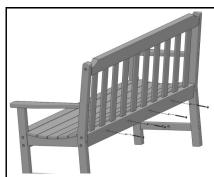
Secure Lower Back Assembly to Seat Assembly using (4) 80MM Hex Lags (3 for 037) thru coun-
