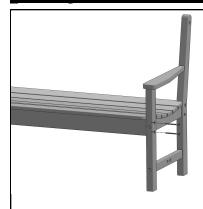
Align Left Side Assembly with seat assembly. Secure using (2) 80MM Hex Lags through the counter-bored
