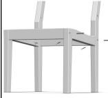
Align Front and Rear Aprons with Front and Rear Legs. Secure with (4) 50mm Hex Lags through
