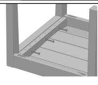
Secure Seat Assembly to Side Assembly using (6) 50mm LAGS.
