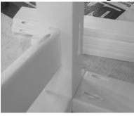
Align back slats in between legs with pocket facing up. Tap into notches on each side of the leg. Secure using (2) 1-1/4" Phillip's head screw. Attach one back slat at a time from the bottom up. Repeat process for all back slats.
