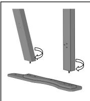
Insert right side Front and Rear Legs into threaded inserts in Right Arm assembly as shown. Turn clock-wise until
