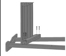
Align counterbored holes in Seat Assembly with threaded inserts in Legs. Attach using (5) 50mm Connect-
