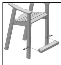
Attach Foot Rest to Front Legs using (4) 80mm Hex Lags thru counter-bored holes in Front Legs. Plug holes with (4) 5/8" Bungs.
