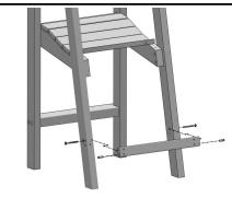
Attach Rear Stretcher to Rear Legs using (2) Nylon D o w e 1 s placed into the larger of
