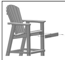
Attach front and rear Seat Aprons by inserting (4) 1 1/4" Phillips Deck Screws into front and rear
