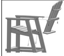
Align Back Assembly with Arms and Seat. Secure upper yoke by inserting (2) 1" Phillips Pan Head
