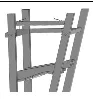
Flip Assembly upside down. Align Side Stretcher with pockets in Front and Rear Legs. Secure using (2) 1 3/4" Phillips Head
