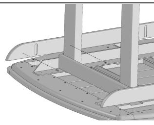
Align Long Aprons with Aluminum Support Brace. Ensure that pockets in Long Apron are aligned with Screws used to attach Short Aprons. Secure using (8) 3/4" Pan Head Screws thru Aluminum Support Brace.
