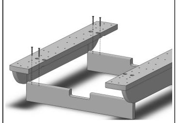
Align slots in long apron assembly with short apron. Secure using (8) 1-1/4" Phillips Head Screws through pilot holes in short aprons.
