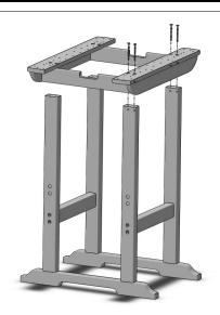
Align counter-bored holes in long apron assembly with Predrilled holes on Legs as shown. Secure using (8) 80mm Hex Lags.
