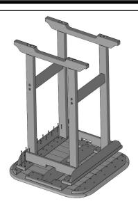
Flip over Base Assembly and align cleats on apron assembly with table top cleats. Secure using (40) 1-1/4" Phillips Head Screws.
