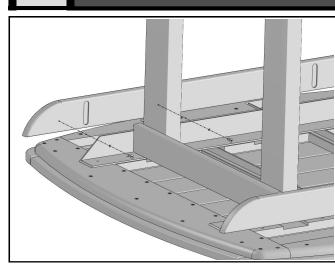
Align Long Aprons with Aluminum Support Brace. Ensure that pockets in Long Apron are aligned with Screws used to attach Short Aprons. Secure using (12) 3/4" Pan Head Screws thru Aluminum Support Brace.
