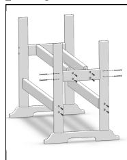
Attach Stretchers to Leg Assemblies using (24) 80mm Hex Lags (8 for Dining Height) as shown. Plug holes with 5/8" Bungs using Rubber Mallet.
