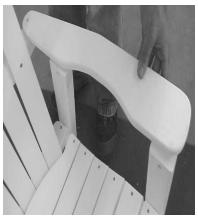
Place Arm Assembly on top of Front Leg and Upper Back Yoke (Left Picture). Align hole in Arm Assembly with the hole located at the top of the Front Leg. Install using (1) 2-3/4" connector bolt through hole in underarm support and though Front Leg with flat & lock washers and nuts (Right Picture). Do not tighten at this time. Repeat process on other side.
